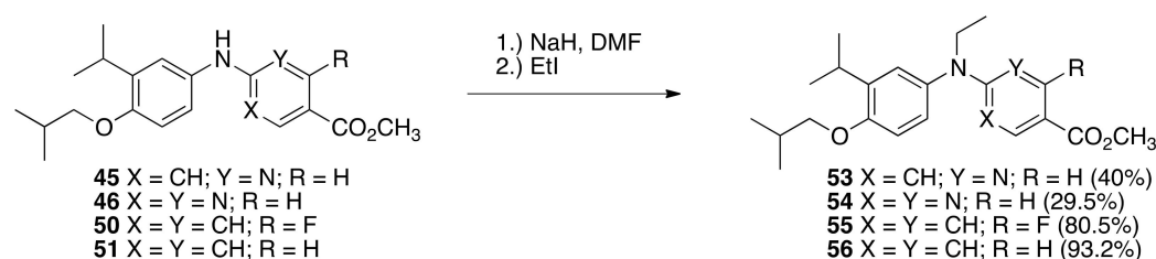
Scheme 3. Synthesis of 53 , 54 , 55 , and 56 from 45 , 46 , 50 , and 51 , respectively.
