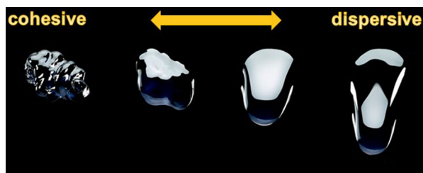
Fig. 1 Classification of OVDs according to their rheological properties
