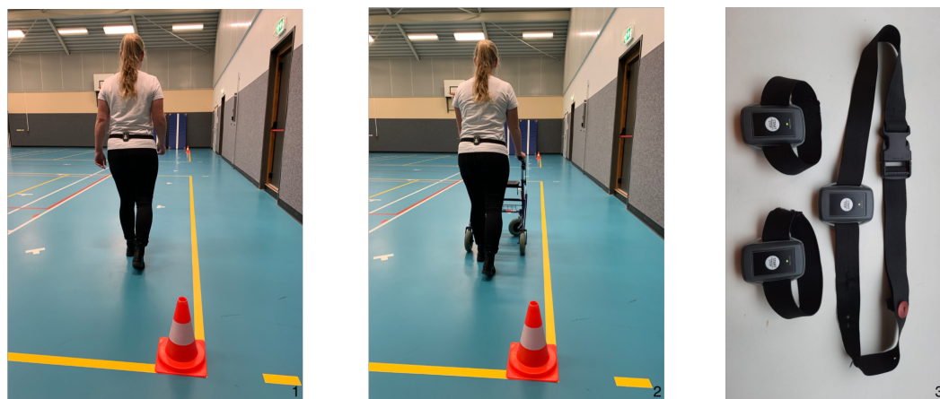
Figure A2. Participants walked on a 14-m path and took right turns around the cones (1,2). The use of a walking aid was optional. The three inertial measurement units were placed at the low back and on top of the left and right feet. Elastic bands were used to hold the sensors in place (3). A measurement was started and stopped by pressing the white start/stop button on the IMUs. After a measurement, the data was stored on the IMU and accessed by connecting the IMU to a computer. The person in the images did not participate in the study.
