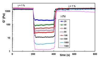
**Figure 7.** Self-healing ability of hybrid hydrogels for increasing strain values illustrated for the sample with  $w_{\rm BSA}$  of 0.5.
