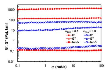
**Figure 2.** Viscoelastic parameters as a function of oscillation frequency, for hybrid hydrogels with  $w_{\rm BSA} = 0.2$  (full red symbol) and  $w_{\rm BSA} = 0.8$  (empty blue symbol) at 37 °C.
