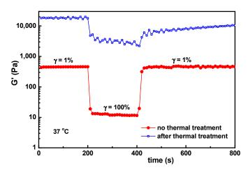
**Figure 10.** The influence of the thermal treatment (sample kept at 70 °C for 1 h and then cooled to 37 °C and thermostated for 1 h) on the self-healing behavior of the hydrogel with  $w_{BSA} = 0.5$ .
