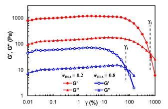
**Figure 1.** Viscoelastic moduli in amplitude sweep tests for two samples of  $w_{\text{BSA}} = 0.2$  and  $w_{\text{BSA}} = 0.8$ .
