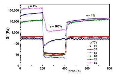
**Figure 9.** Temperature influence on the self-healing behavior of hybrid hydrogels for the sample with  $w_{\rm BSA} = 0.5$  submitted to successive step strains of 1%–100%–1%.
