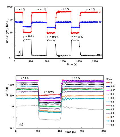
**Figure 6.** Self-healing behavior of hydrogels illustrated through consecutive step strain measurements at 37 °C: (a) G', G'' and  $\tan\delta$  for the hydrogel with  $w_{\rm BSA}=0.5$  during several successive runs of low (1%) and high (100%) strains; (b) G' for different polymer/protein compositions during the first run of strain (1%– $\uparrow$  100%– $\downarrow$  1%).
