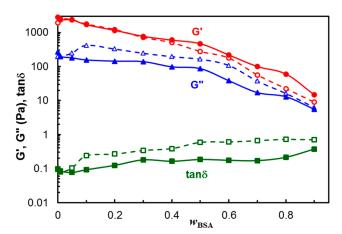
**Figure 3.** Viscoelastic parameters as a function of  $w_{BSA}$  for PVA/HPC and hybrid polymer/BSA hydrogels after 3 freezing thawing cycles,  $\omega = 1$  rad/s,  $\gamma = 1\%$ , at 25 °C (empty symbol, dashed line) and 37 °C (full symbol, continuous line). The lines are a guide to the eye.
