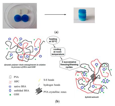
**Figure 5.** (a) Macroscopic image showing the self-healing behavior of hybrid hydrogels ( $w_{BSA} = 0.5$ ). (b) Schematic presentation of hybrid hydrogel formation.
