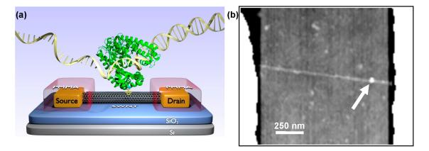
**Figure 1.** (a) Schematic of a single-walled carbon nanotube field effect transistor (SWNT-FET) functionalized with a single copy of a protein. This device depicts the Klenow Fragment of DNA polymerase I converting a single-stranded DNA template into a double-stranded helix. A pyrene-maleimide (**yellow**) is shown linking the protein to the SWNT. (b) Atomic force microscopy image of a typical SWNT-FET device after functionalization confirms attachment of a single protein (**arrow**).
