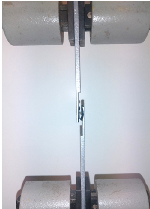
Figure 6. View of the sample after the shear test.
