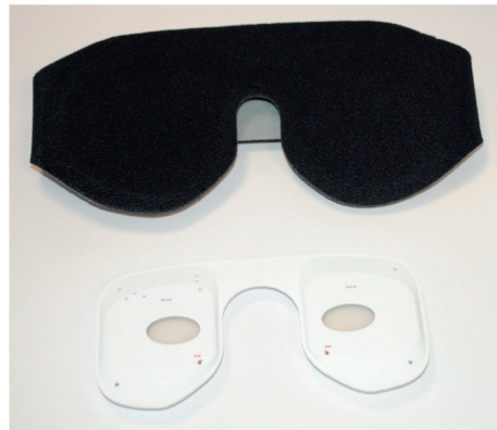
FIGURE 1: Picture of the black fabric mask and the white plastic pod housing the OLED lighting that make up Noctura 400.
