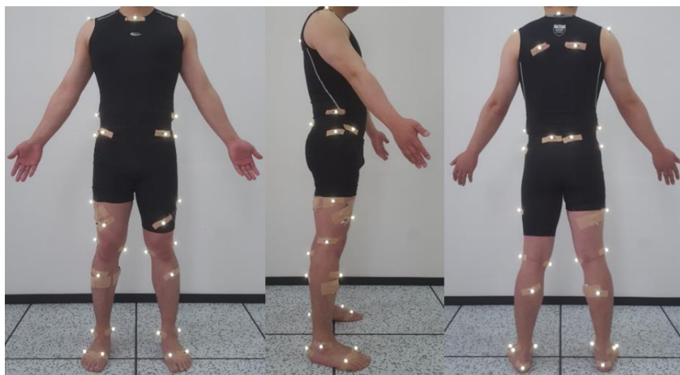
Figure 4. Location of the reflective motion capture markers.
