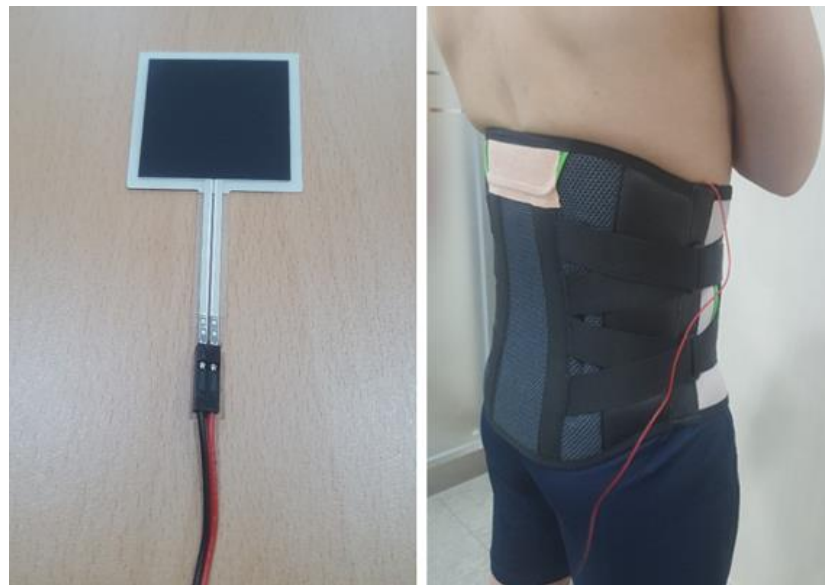
Figure 1. Measurement of the pressure of the lumbar belt using a force-sensing resistor.
