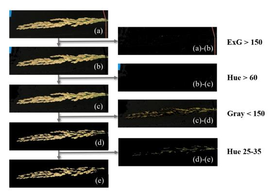
**Figure 9.** Background removal process included the (a) ROI image, (b) ROI image with ribbon removal, (c) sample card removal from image (b), (d) shadow removal from image (c), and (e) stem removal from image (d).
