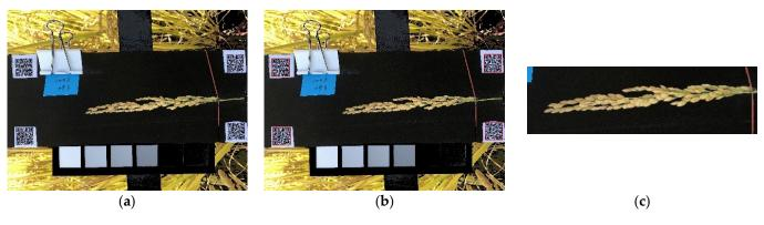
Figure 8. ROI cropped display. Corrected image (a), QR code detection (b), and ROI area (c).
