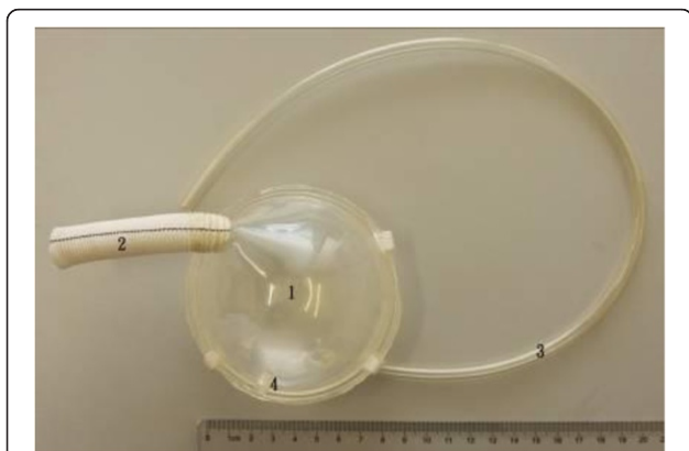
Fig. 1 Photograph of an extra-thorax paraaortic counterpulsation device (ETPACD). The ETPACD sac fills with 120-ml (a 65-ml stroke) blood volume (1) during ventricular systole and empties during ventricular diastole through a single valveless cannula (2). The diaphragm is pneumatically driven by the console through a gas line (3) and the gas outlet (4)
