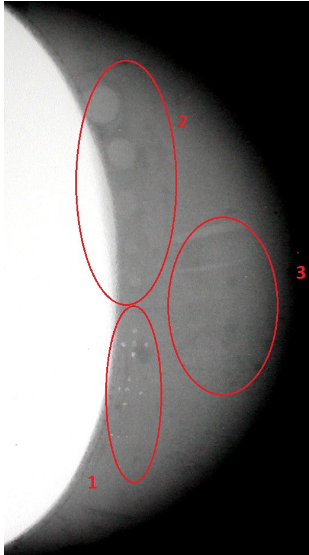
FIG. 5. Image of the proposed phantom containing the silicone implant and the inserted artifacts: microcalcifications (detail 1), tumor masses (detail 2) and fibers (detail 3).
