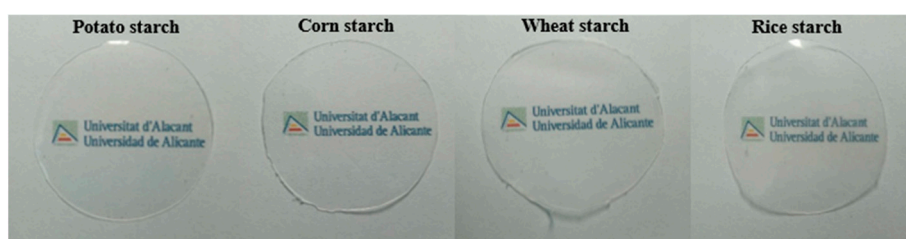
Figure 2. Visual aspect of films obtained from potato, corn, wheat, and rice starch.
