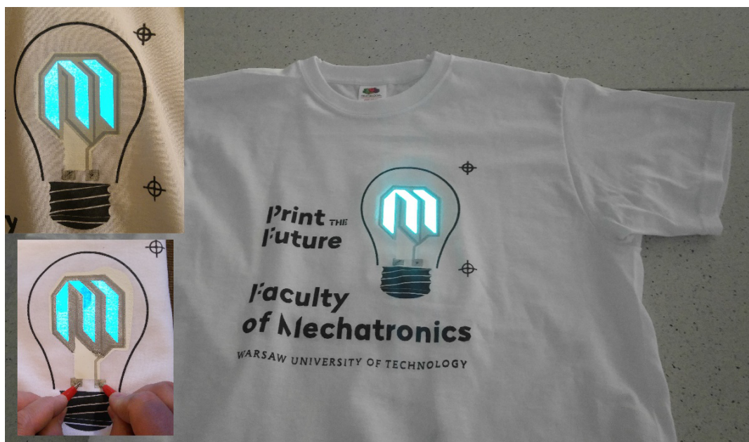
Figure 3. T-shirt with printed electroluminescent display. Upper left corner: Electroluminescent (EL) structure with carbon nanotube electrode, lower left corner: EL structure with an ATO-based electrode.
