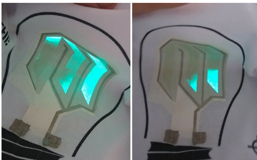
Figure 4. Visible degradation of two exemplary electroluminescent structures with an ATO-based electrode after first wash.
