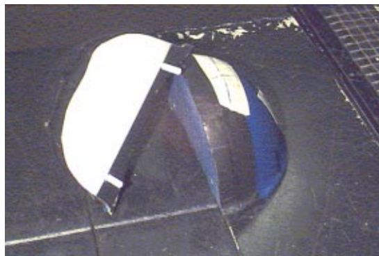
FIG. 3. (Color) Breast phantom cut in half and showing the polyethylene filler and dowel. The film was cut to the size of the white area of the filler and placed between the filler and the opposite breast half. The positions of the isocentric positioning lasers are indicated by the crosshairs on the phantom.
