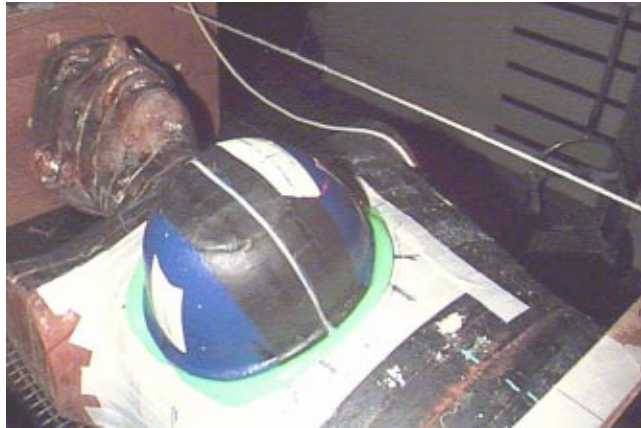
FIG. 1. (Color) Positioning of the breast phantom on the anthropomorphic phantom. Crosshairs and laser lines are indicated on the phantoms. The markings were necessary on both phantoms to ensure that they were positioned correctly (i.e., the anthropomorphic phantom on the treatment couch and the breast phantom on the anthropomorphic phantom).
