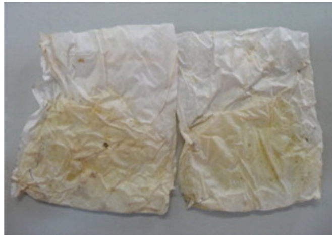
Figure 4. Pictograph of a PLA Biophan 121 pouches after HP sterilization (700 MPa at 115 °C for 5 min) containing solid carrots as packaged foodstuff, reprinted with permission from Ref. [54], copyright (2022) Elsevier.
