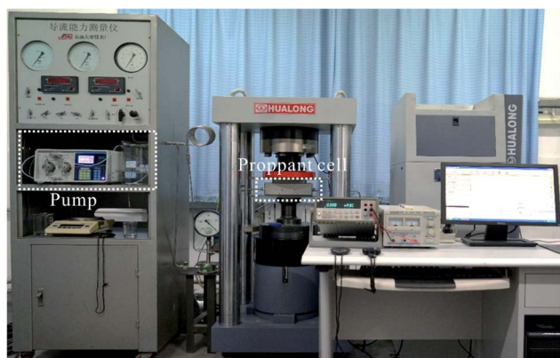
Fig. 6 Conductivity test device.
