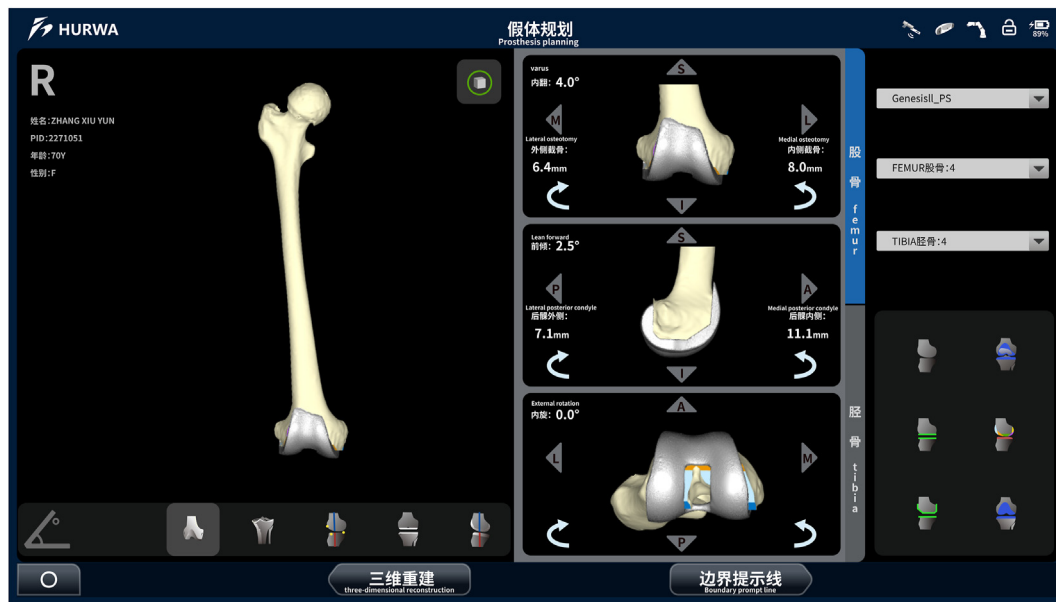
Figure 2. Preoperatively planned position and posture of a femoral component by the HURWA robot-assisted TKA system.
