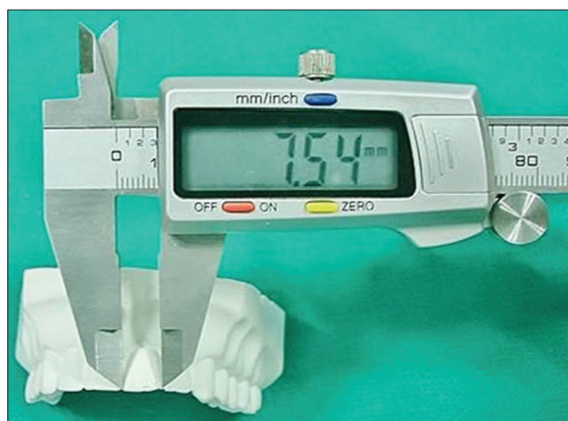
Figure 2: Mesiodistal crown widths of the maxillary anterior permanent six teeth using vernier calliper
