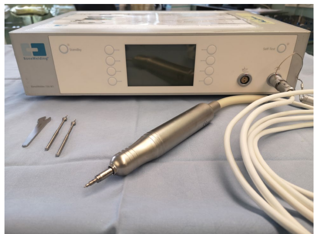
Fig. 1 Hand piece, drill bits and BoneWelding® melting machine
