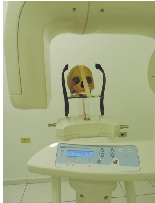
Fig. 2. Acrylic device designed to position the anatomical pieces during cone-beam computed tomography scanning.
