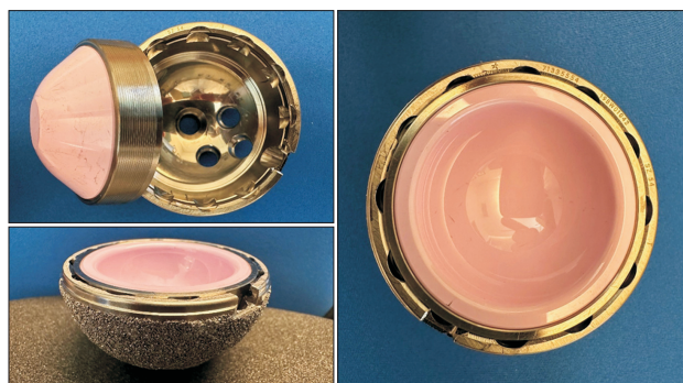
Fig. 4. Accurate alignment position of a delta ceramic liner with a titanium locking band into an 18° inner taper locking angle cementless hemispherical porous-coated acetabular shell. No visible overhang of the titanium metal part from the acetabular shell.
