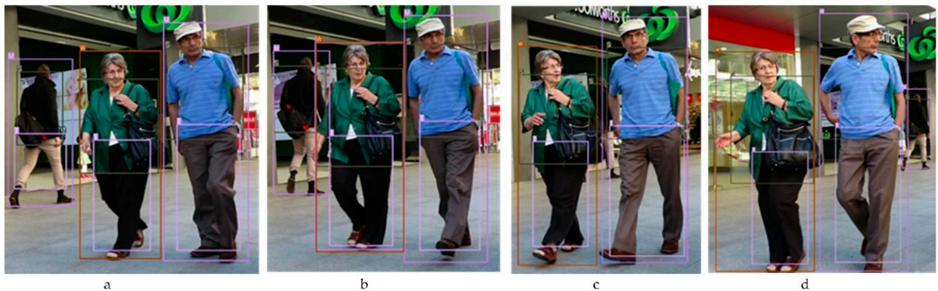
Figure 7. Four images taken from our detection outputs to demonstrate the occlusion phases. The original image is taken from the MOTChalleng dataset [28]. Before occlusion state (a), in occlusion state (b,c), and after occlusion state (d).
