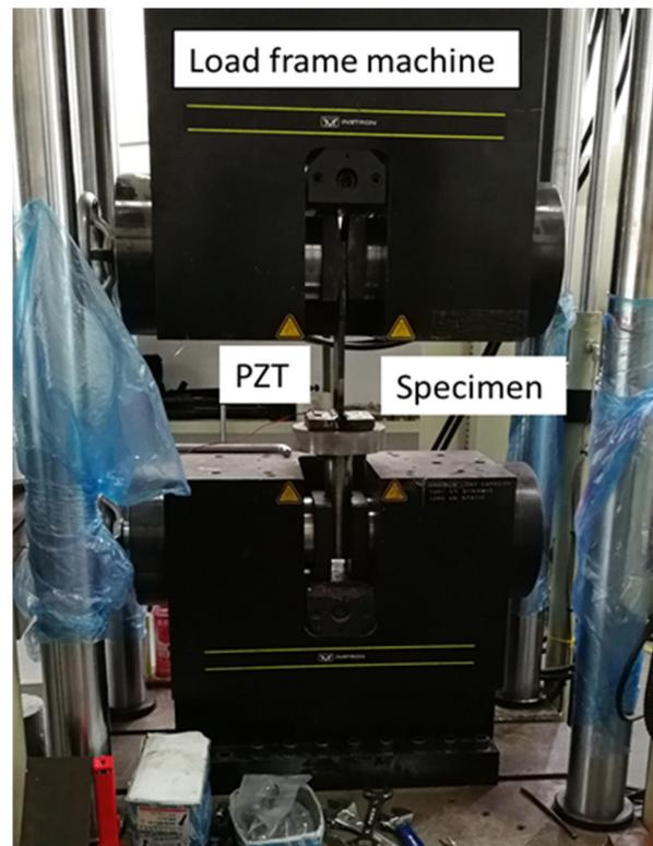
Figure 6. Experimental arrangement.
