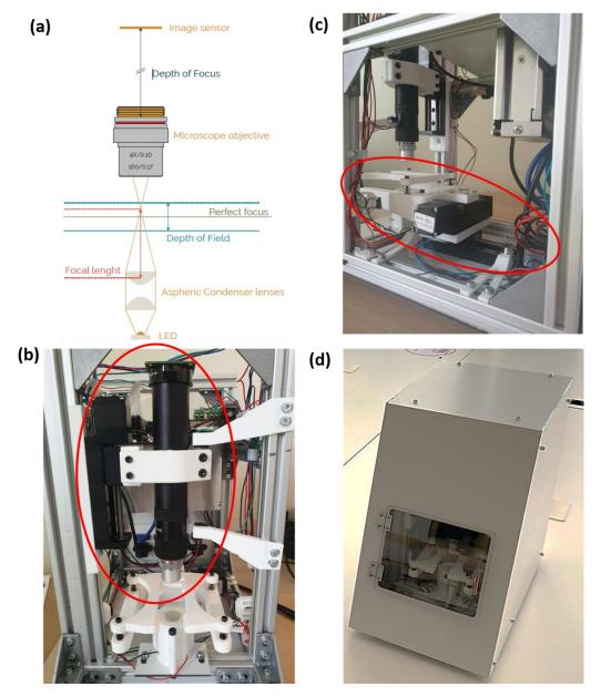
**Figure 1.** (a) Schematic diagram of the Schistoscope optical train (b) Region of interest showing the Z-axis consisting of a mechanical slider and optical setup (c) Region of interest showing the sample stage mounted on the X and Y slider mechanism (d) Exterior of the Schistoscope device (embodiment).
