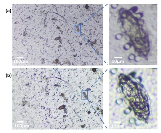
**Figure 5.** Optical performance of the Schistoscope. (**a**) Schistoscope (NA 0.1) and (**b**) conventional microscope (NA 0.25) images of fecal smear containing *Schistosoma haematobium* eggs. Enlarged ROIs show similar optical qualities.
