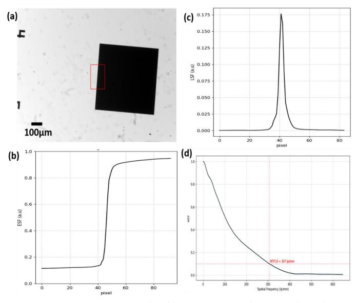
**Figure 4.** Resolution limit of the Schistoscope. (a) Slanted-edge image with selected rectangular region of interest (b) Edge spread function curve (c) Line spread function curve (d) Modulation transfer function curve with a resolution limit of 307 lp/mm.
