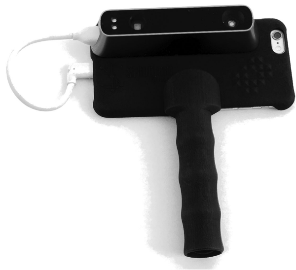
FIGURE 2 3D imaging system with phone. Prototype hardware setup is from Body Surface Translations, Inc. A structure sensor 3D scanner is connected to a phone. 3D, 3-dimensional.
