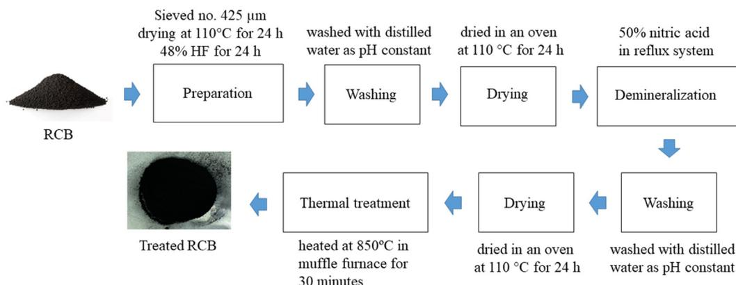
**Figure 1.** Flowchart of the chemical treatment of RCB.
