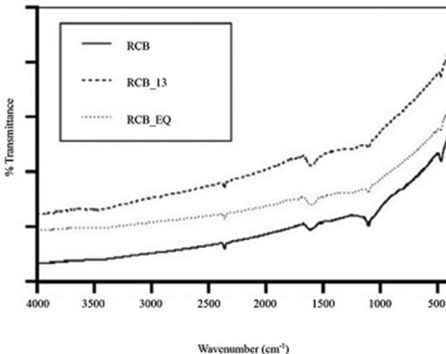
Figure 8. FTIR spectra of carbon black.
