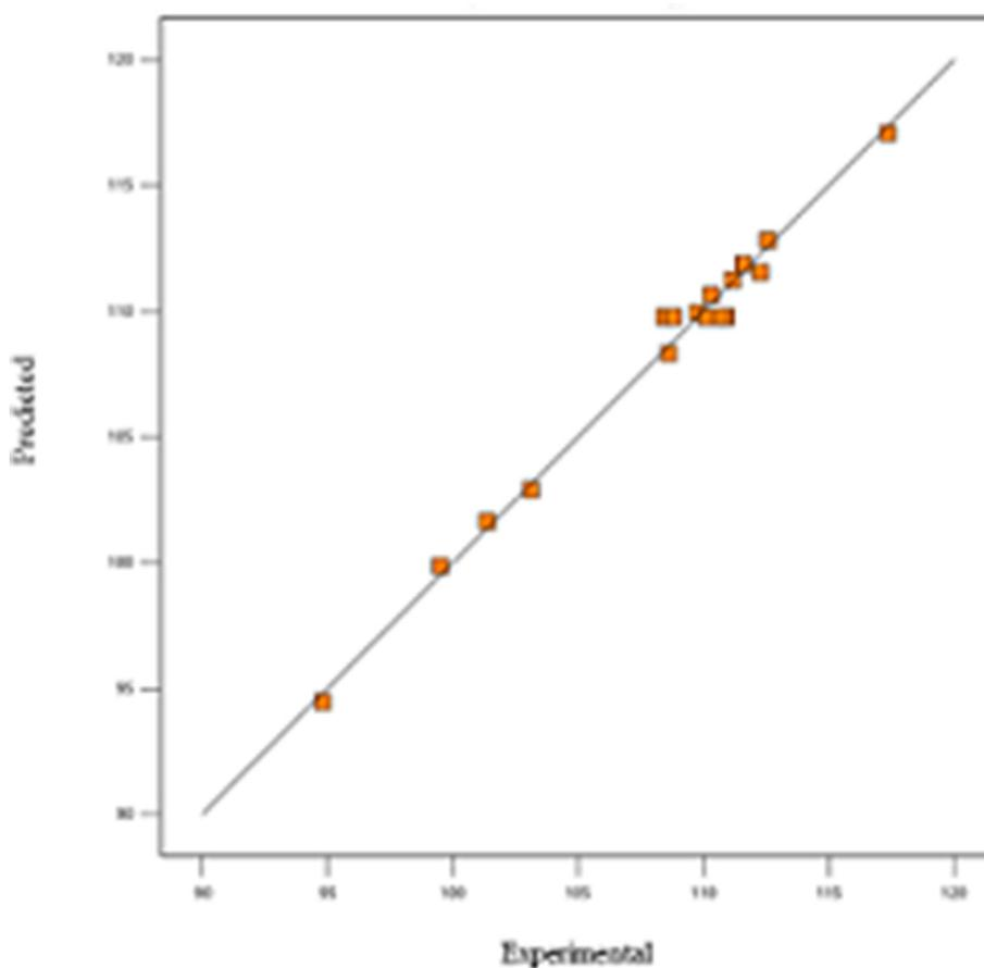
**Figure 2.** Predicted versus experimental iodine numbers of carbon black.
