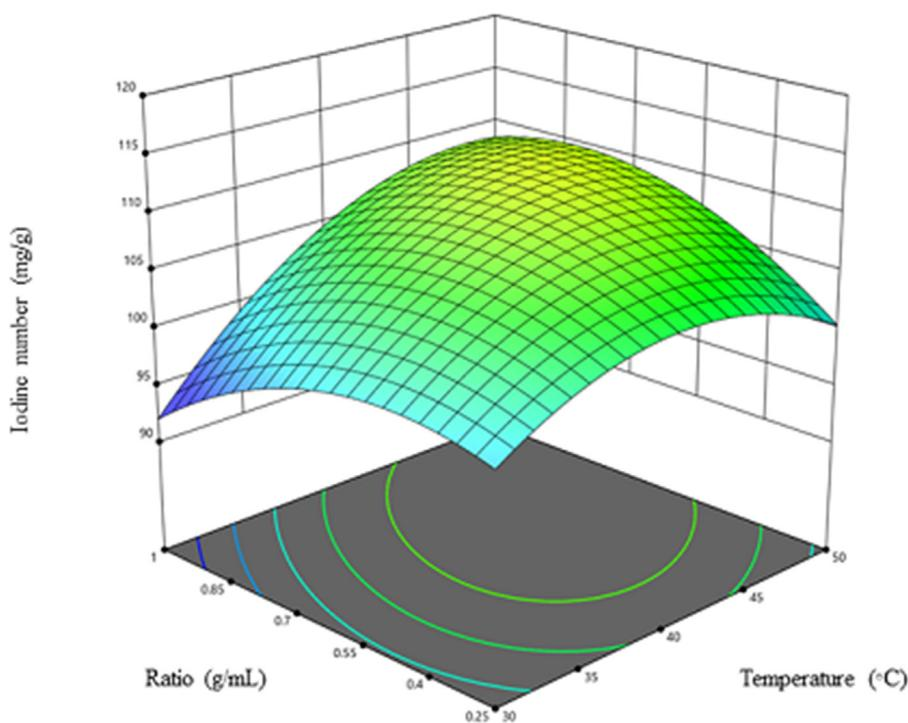
**Figure 3.** Effect of the interaction between temperature (A) and ration (B) on iodine number.
