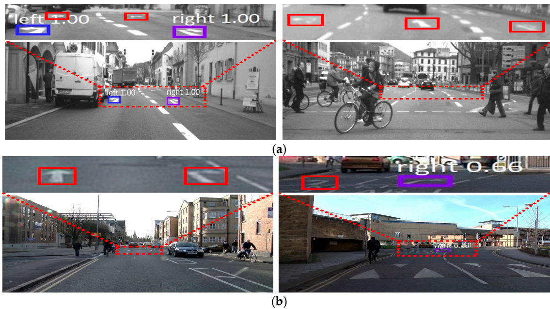
Figure 12. Examples of incorrect detection and classifications. (a) Test2 of the Daimler dataset. (b) Seq06R0 of the Cambridge dataset. In (a,b), the red colored boxes with solid lines indicate false negatives whereas the boxes of other colors represent true positives.
