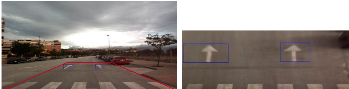
Figure 14. Examples of the original (left image) and its corresponding IPM images (right image).
