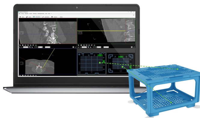
Figure 1. The CNS system consisting of the PC on the right, and software on the left. The software displays the standard MPR views in coronal, sagittal and axial views. Shown here is an example infiltration at the lumbar level. The chosen trajectory of the virtual needle is shown as a highlighted yellow cross-hair marker which can be freely moved. Based on the trajectory of the needle, the corresponding coordinates in the upper-left and lower-right templates are highlighted by the software. The physical puncture needle is then inserted through these holes.
