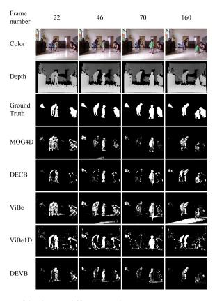
**Figure 4.** Comparison of background/foreground segmentation images generated by various background subtraction techniques for four frames taken from the *child\_no1* sequence without morphological filtering. The segmented images produced by our method are the closest to the ground-truth references. MOG4D: 4D version of Mixture of Gaussians. DECB: Depth-Extended Codebook. ViBe: visual background extractor. ViBe1D: ViBe based only on depth. DEVB: Depth-Extended ViBe.
