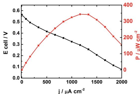
Fig. 5 Electrochemical performances of a DEFC at  $25 \text{ }^\circ\text{C}$  using Pt<sub>50</sub>Rh<sub>50</sub>/C ( $0.13 \text{ mg cm}^{-2}$ ) and PdSe/C ( $0.13 \text{ mg cm}^{-2}$ ) as anode and cathode catalysts, respectively; the anodic compartment contains  $1 \text{ mol L}^{-1} \text{ NaOH}$  and  $1 \text{ mol L}^{-1}$  ethanol separated to the cathodic one by an AEM from Fumatech.
