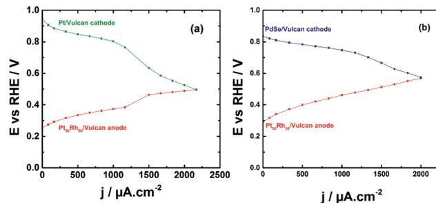
Fig. 4  $E$ - $j$  polarizations curves obtained at the electrodes of a DEFC operating at room temperature and in alkaline medium. (a) (–) Pt<sub>50</sub>Rh<sub>50</sub>/C/ $1.0 \text{ mol L}^{-1}$  ethanol/ $1.0 \text{ mol L}^{-1}$  NaOH, O<sub>2</sub>/Pt/C (+); (b) (–) Pt<sub>50</sub>Rh<sub>50</sub>/C/ $1.0 \text{ mol L}^{-1}$  ethanol/ $1.0 \text{ mol L}^{-1}$  NaOH, O<sub>2</sub>/PdSe/C (+).
