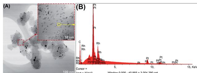
**Fig. 2** (A) TEM images for Pt<sub>50</sub>Rh<sub>50</sub>/C material. (B) EDX spectra of Pt<sub>50</sub>Rh<sub>50</sub>/C particle.
