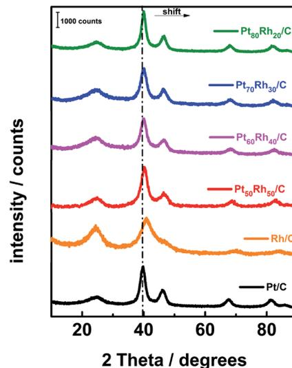
Fig. 1 XRD patterns of the carbon supported Pt<sub>x</sub>Rh<sub>y</sub> materials prepared from the revisited BAE method.
