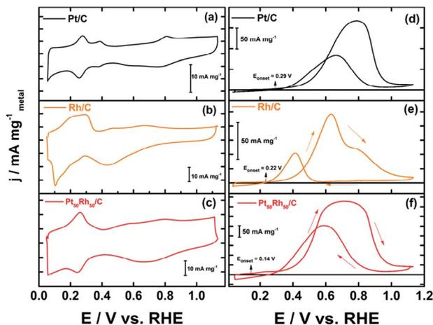
Fig. 3 Voltammograms (CVs) of Pt and Rh based electrode materials prepared from the revisited BAE route. These CVs were recorded at room temperature and  $10 \text{ mV s}^{-1}$  and in  $1 \text{ mol L}^{-1} \text{ NaOH}$ , in the absence (a, b and c) and the presence of  $0.2 \text{ mol L}^{-1}$  ethanol (d, e and f).
