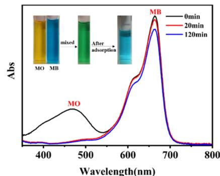
Fig. 6 Dye selectivity of ICOF with mixed dye (MB and MO) initial concentration: 20 mg L<sup>-1</sup>; adsorbent mass: 2 mg; volume: 6 mL.
