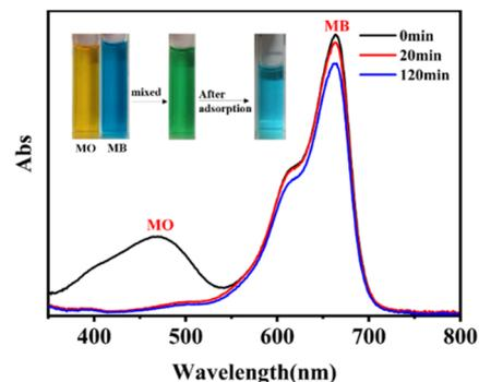
Fig. 6 Dye selectivity of ICOF with mixed dye (MB and MO) initial concentration:  $20 \text{ mg L}^{-1}$ ; adsorbent mass: 2 mg; volume: 6 mL.
