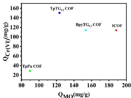
Fig. 7 The adsorption capacity of different adsorbents for MO and Cr(vi) in the binary mixed pollutant system (initial concentration: 200 mg L<sup>-1</sup>; adsorbent dose: 3 mg; volume: 6 mL; pH: 3; temperature: 310 K).
