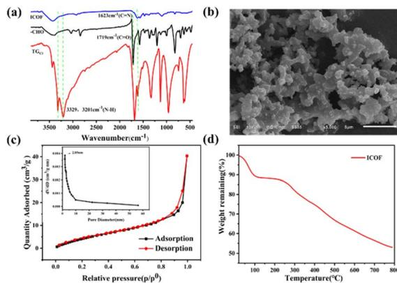
Fig. 2 (a) FTIR spectrum of ICOF, reactants –CHO and TGCl. (b) SEM images for ICOF. (c) N<sub>2</sub> adsorption isotherm (77 K) and pore size distribution profiles. (d) TGA curves of ICOF.
