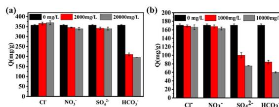
Fig. 4 Influence of co-ions on the elimination of MO and Cr(vi) on ICOF. (a) MO ( $C_{\text{MO}} = 200 \text{ mg L}^{-1}$  and  $C_{\text{M}} = 0, 2000, \text{ or } 20\,000 \text{ mg L}^{-1}$  each; adsorbent dose: 3 mg; volume: 6 mL; pH: 3; temperature: 310 K). (b) Cr(vi) ( $C_{\text{Cr(vi)}} = 100 \text{ mg L}^{-1}$  and  $C_{\text{M}} = 0, 1000, \text{ or } 10\,000 \text{ mg L}^{-1}$  each; adsorbent dose: 3 mg; volume: 6 mL; pH: 2; temperature: 310 K).
