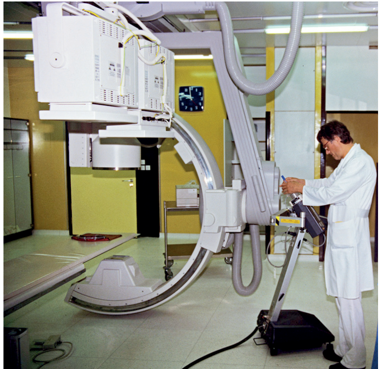
FIGURE 15. Philips-Integris C for digital subtraction angiography (1993–2009) (Marijan Klemenc, Radiol. Ing. )
