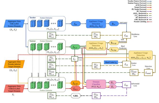
**Figure 1.** A detailed overall configuration diagram of the proposed semi-supervised domain adaptation for multi-label classification on nonintrusive load monitoring.
