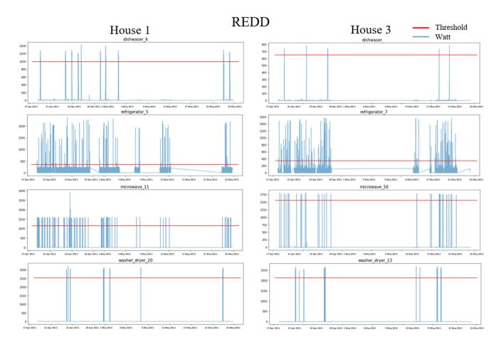
**Figure 4.** Power usage and ON thresholds for House 1 and House 3 in the REDD dataset.
