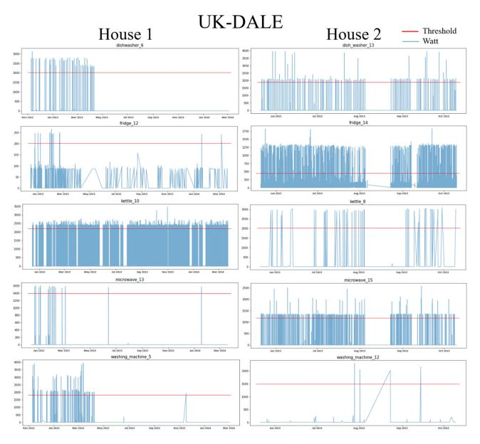
Figure 3. Power Usage and ON Thresholds for House 1 and House 2 in the UK-DALE dataset.
