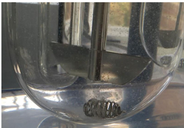
Fig. 6 An image of LP-8 liqui-pellet disintegrate explosively in acidic dissolution medium. Note the small white specks are fragments of the liqui-pellet
