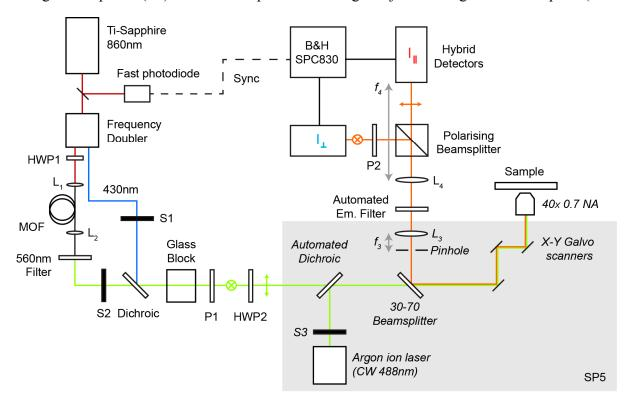
**Figure 5.** Schematic of the multiplexed polarisation resolved microscope described in the text. Components inside the grey area and labelled in italics are internal to the SP5 confocal microscope. Abbreviations used: HWP, half wave plate; S, shutter, P, polariser, L, lens. The focal lengths of lenses  $L_3$  and  $L_3$  are labelled  $f_3$  and  $f_4$ , respectively.
