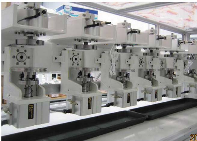
Figure 2. Six-Station Prosim 2 Hip Simulator (Simsol, Stockport, UK). doi:10.1371/journal.pone.0045786.g002
