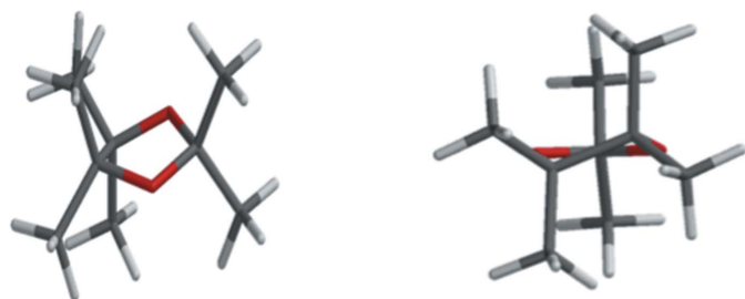
Figure 6 Perspective views of dioxolane ring with methyl groups as calculated with Spartan . Left: viewed as distorted envelope. Right: viewed as twist.
