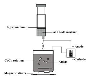
Figure 1. The device used in the microencapsulation process by means of the complex coacervation method. doi:10.1371/journal.pone.0061129.g001
