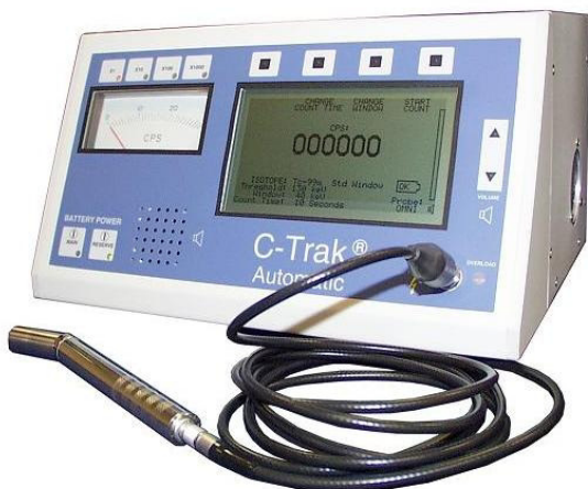
Figure 1 A basic gamma probe system. Control unit and probe. (Courtesy of Care Wise Medical Products Corp., CA, US).
