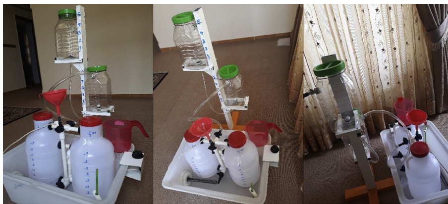
Figure 1. Bioreactor pictures made for the biological removal of iron and sulfate from wastewater.
