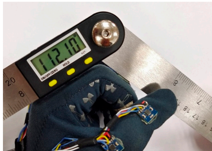
Figure 16. Comparison of the measured angle between data glove and digital goniometer.
