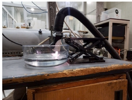
Fig. 2. Exposing distilled water to gliding arc plasma produced by Plasmatek-15B
