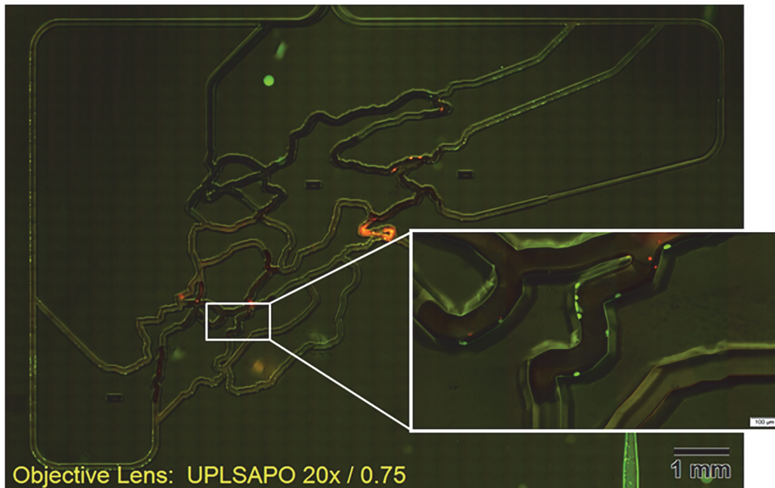
Fig 10. Endothelial and fibrosarcoma cells in the whole microfluidic channel. Endothelial cells (emitting green fluorescence) and fibrosarcoma cells (emitting red fluorescence) in the whole microfluidic device. The image was generated by superimposing two-color fluorescence images. The 20× objective lens (NA 0.75) was used.
