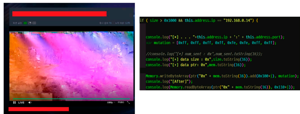
Figure A7. Example of DoS attack through video data tempering (picture distortion).
