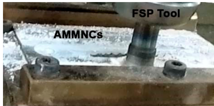
Figure 1. Friction Stir Processing (FSP) using vertical milling machine with fixture installation.
