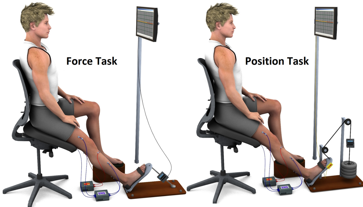
Fig 1. Schematic representation of the experimental setup. Subject positioned during the force (left part) and position tasks (right part). In the force task (FT), the right foot was strapped to a pedal connected to a force transducer and the subjects had the ongoing plantarflexion force as visual feedback (signals from the force transducer). In the position task (PT), the pedal was attached to the load via a pulley system and visual feedback of the ankle angle (signals from the accelerometer, depicted at the right side of the base of the pedal) was provided. The scheme shows the location of recording and stimulation electrodes (connected with blue and red wires, respectively) for posterior tibial nerve and common peroneal nerve stimulation and for soleus, tibialis anterior, semitendinosus, and vastus lateralis EMG acquisition.
