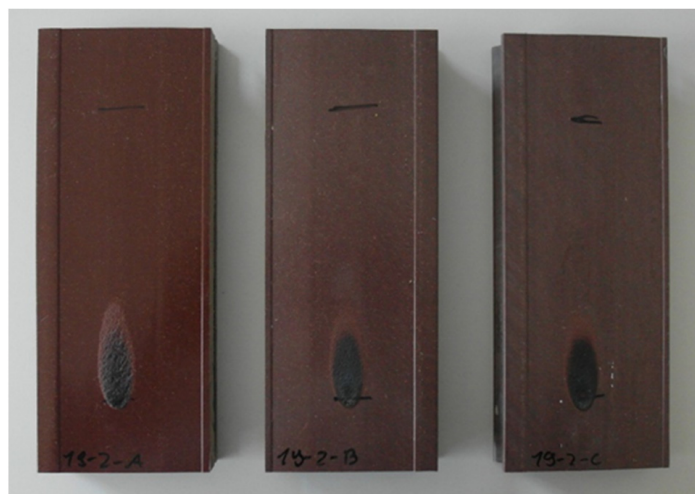
Figure 3. Hollow core profiles after the single flame source test (EN ISO 11925-2). From left to right: reference without FR, profiles with Budit 669, and profiles with FR CROS 490. Horizontal line on profiles indicates 150 mm-mark (vertical flame spread within 60 s after start of the flame treatment shall not be more than 150 mm).
