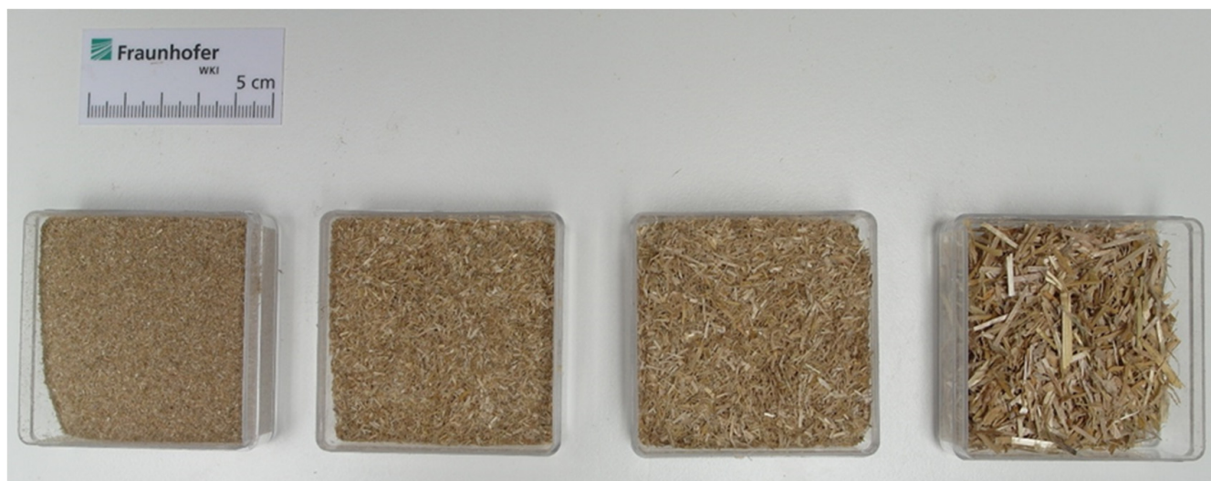
Figure 2. Particle size fractions after sieving. From left to right: 0.6–1.25 mm; 1.25–3.15 mm; 3.15–5 mm; >5 mm. Fraction < 0.6 mm not shown.
