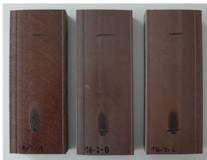
Figure 4. Solid profiles after the single flame source test (EN ISO 11925-2). From left to right: reference without FR, profiles with Budit 669, and profiles with FR CROS 490. Horizontal line on profiles indicates 150 mm-mark (vertical flame spread within 60 s after start of the flame treatment shall not be more than 150 mm).
