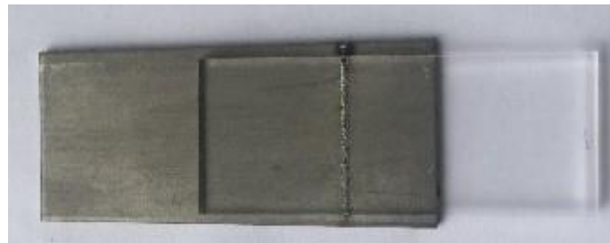
Figure 4. Welding between titanium alloy and high borosilicate glass.
