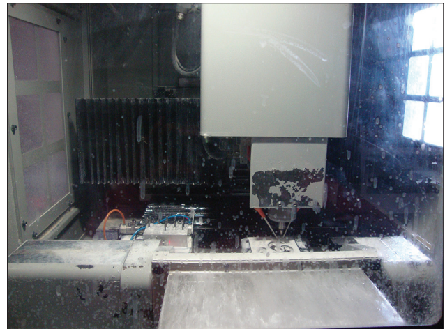
Figure 2: Metal milling of titanium blank for abutment copings
