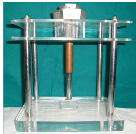
Figure 4: Alignment apparatus applying a weight of 750 g to the bonded specimens
