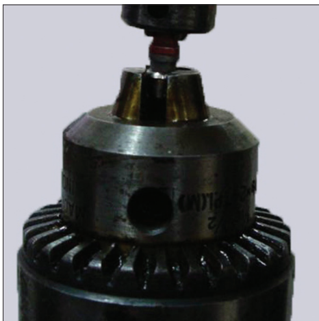
Figure 5: Pull-off test for determination of bonding strength
