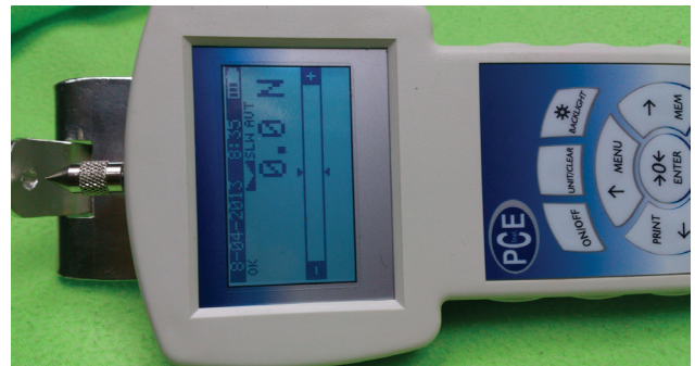
Figure 2. Dynamometer with a specifically designed force transducer of the lower jaw bite (original photograph taken by the author)
